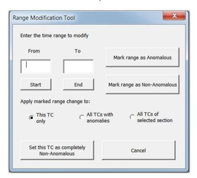
The range modification can be made to only the channel selected, all the channels assigned to the selected section with identified anomalies (as listed on the Anomalous Data page), or to all channels assigned to section. The radar buttons are used to select the required option.
