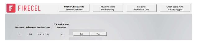
Each section in the test is listed, along with the TC number of any valid thermocouples which FIRECEL has detected any anomalous data in (whether it is at one single time step, or all).
