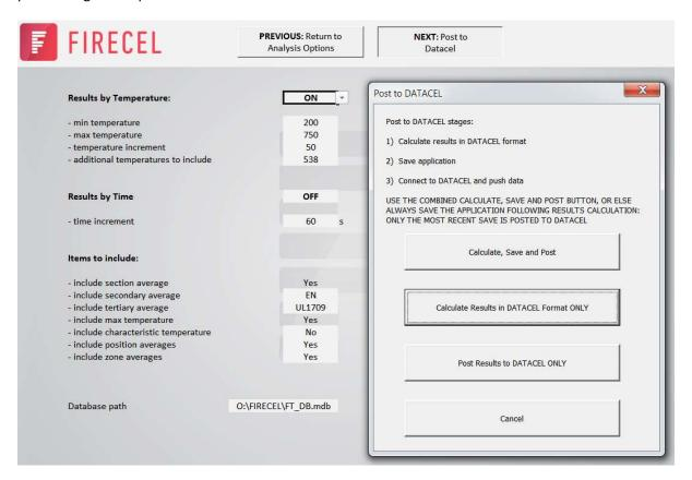
To perform all calculate, save and post steps in one go, users should click *Calculate, Save and Post*. A save file dialogues box will be displayed mid-way through the process prompting user input. The options are also given for advanced users to calculate only and post only, allowing check of calculated data before manually saving and posting.
