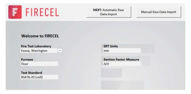
The user can choose to automatically import raw data and allow FIRECEL to choose the layout and detailed settings, or to manually import data and review the detailed settings themselves. If *Automatic Raw Data Import* is selected the user may be prompted to navigate to the appropriate file and select the relevant worksheet (if more than one worksheet with data is detected in the raw data
